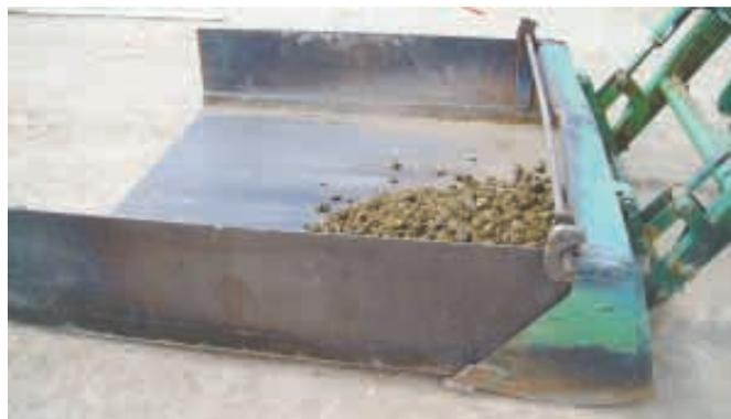
Steel basket hooks inside loader bucket to greatly increase its carrying capacity.
