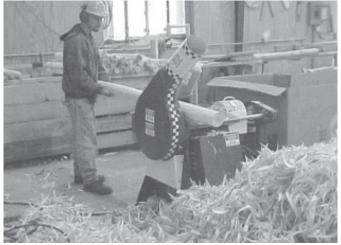
German-style log peeler removes bark from logs that are used for railing, furniture and log home construction.
