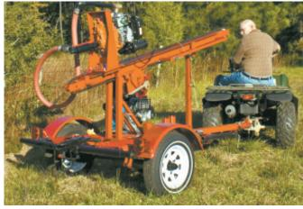
ATV-sized, trailer-mounted well-drilling rig goes anywhere and drills as deep as 300 ft.
