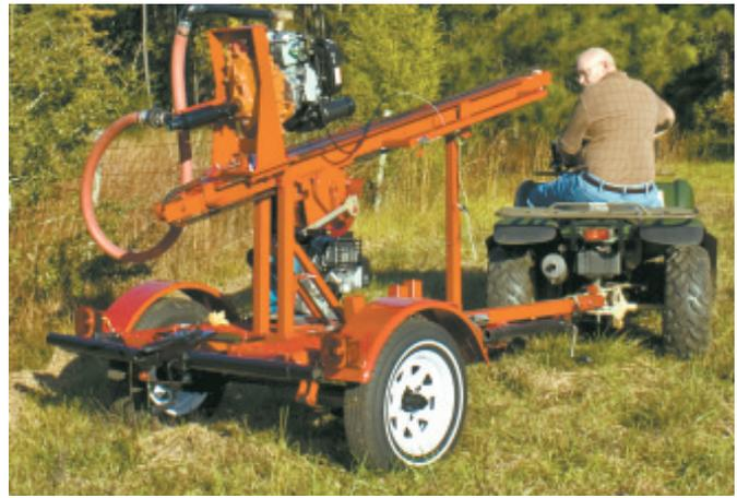
ATV-sized, trailer-mounted well-drilling rig goes anywhere and drills as deep as 300 ft.
