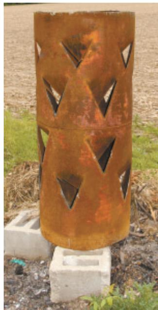
V-shaped tabs, bent in toward center of pipe, hold up trash until it's mostly burned up. The V-slots also give trash plenty of combustion air.
