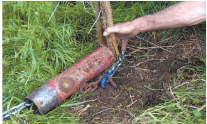
"Brush strangler" is a piece of thick-walled pipe with a short length of chain welded to the side. Pipe bites into brush to rip it out of the ground.
