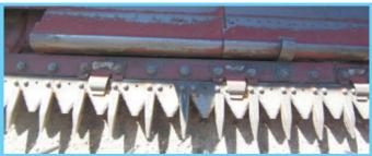
Photo shows original flex head platform before it's rebuilt.
