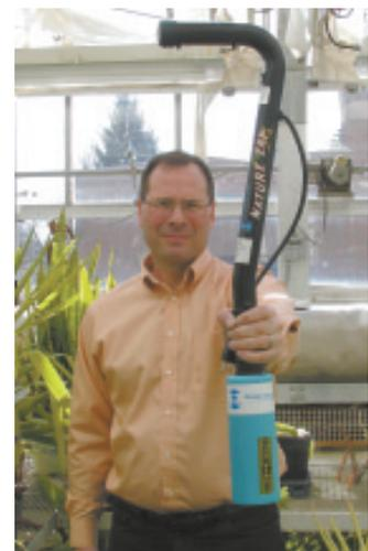
**Electric-powered tool kills weeds by overheating cells at base of stem. "When you press the heating element probe into the plant base, it actually explodes cells," says importer Jon Jackson.**
