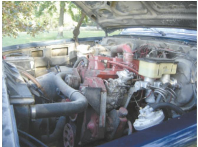
**Bruce Basinger replaced the 350 V-8 engine in his 1984 Chevy pickup with a Cummins 4-cyl. engine.**
