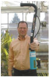
Electric-powered tool kills weeds by overheating cells at base of stem. "When you press the heating element probe into the plant base, it actually explodes cells," says importer Jon Jackson.
