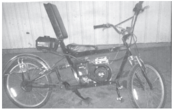
He recently mounted a 6 1/2 hp pressure washing engine on a mountain bike. A torque converter purchased from Northern Hydraulics serves as the drive and clutch.
