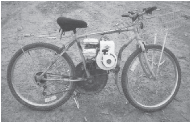
Ron Flynn equipped his first motorized bike with a 2 hp Briggs & Stratton engine.
