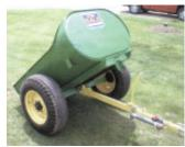
Trailer's dump is activated by pulling a lever mounted on the tongue.
