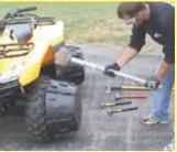
Replaceable rubberized traction blades fit into slots on hubs.
