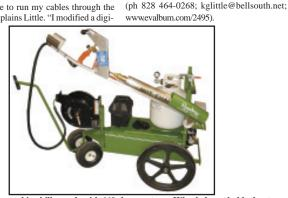
Green Steam machine kills weeds with 660-degree steam. Wheeled cart holds the steam thrower gun, 7-gal. water tank, 20-lb. propane bottle, and battery.
