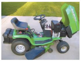
Gary Little converted his 1997 Deere Sabre riding mower to electric power, replacing the 16 hp engine with an Etek DC motor from Briggs & Stratton.
