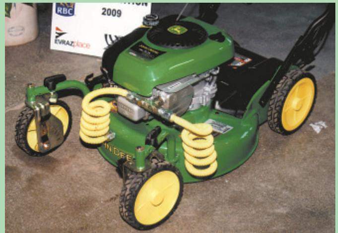
Exhaust gas on this Deere mower is injected under the deck after running through cooling coils.
