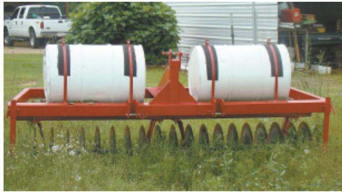
Two 55-gal. barrels mounted on top of aerator frame are equipped with faucets at their bottoms, making it easy to add or reduce weight by adjusting water levels.
