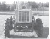
The Jeep tractor's cab consists of 2 1/2-in. galvanized pipe with a sunshade top made from the shell of a clothes dryer. The windshield was salvaged from a 1974 motor home, as was the operator's seat. The hood over the motor is the shell of an old refrigerator, hinging forward over the radiator. The large radiator was salvaged from a Dodge pickup truck. With the help of a 24-in. fan from a big diesel engine, the radiator has kept the rig cool even when plowing in 100 degree temperatures.
