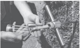
Temperature probe works together with computer software.A removable, battery-powered data logger on back plugs into the USB port on your computer.
