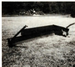
L-shaped blade is 7½ ft. long, 19 in. high.
