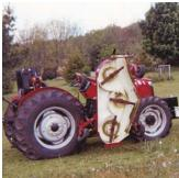
An ATV winch that operates off the tractor battery is used to fold the mower upright for transport.
