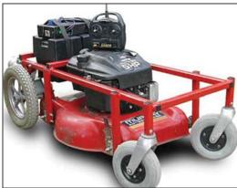
Using website plans you can build your own radiocontrolled lawn mower for less than \$500. Mower is powered by the motor and batteries from an electric wheelchair.
