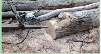
Struble cuts 8-ft. logs in two and drills a 4-in. deep, 1-in. dia. hole in one end of each log.
