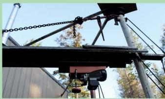
Tower-style log loader consists of a pivoting center post with a 10-ft. boom and a traveling hoist. Struble uses a hand-held remote control to activate hoist to drop "log handle" to log.
