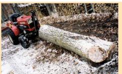
Dan Jacobson's home-built log skidder mounts on front of his Yanmar 18 hp garden tractor.
