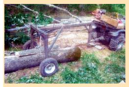
Mark Folz built this log skidder to pull behind his ATV. By using mostly scrap metal he kept the cost down to about \$300.
