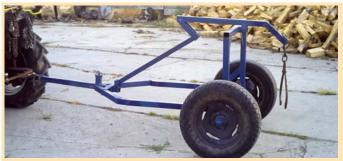
Innovative log arch pins to tractor drawbar and uses its own tongue to lift front end of log off the ground.
