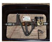
When water pressure drops, a triggerrelease spring closes a valve and flips up the spring-loaded stick like a tip-up.
