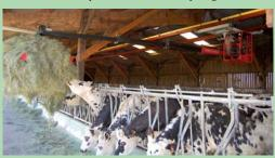
Crane's arm extends up to 30 ft. to grab more than 800 lbs. of hay at a time and place it in front of cows in tie stalls.
