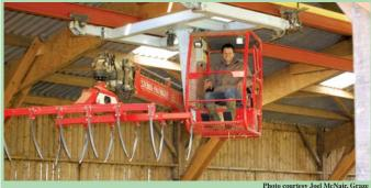
Electric crane consists of a hayfork on a track. It's used to move 40 to 50 percent moisture hay from transport wagons to drying bins.
