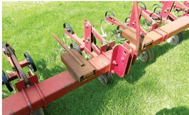
Forks on loader slip into a pair of box tubes welded onto the top of cultivator toolbar.
