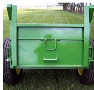
Trailer's box comes with a spring-loaded latch. When released, box manually tilts overcenter.
