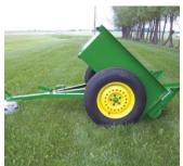
Heavy duty ATV dump trailer is designed to haul up to 1 ton of rocks behind an ATV.
