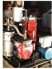
All kinds of waste can be used to power the new "Power Pallet". A gasifier control unit automatically adjusts the fuel-air mix for the material being burned.
