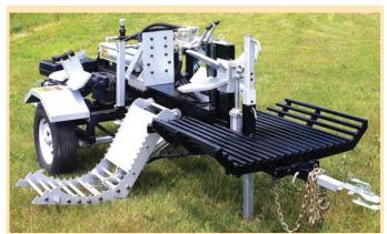
Log-gripping pusher plate on this splitter keeps log from slipping out when splitting firewood.
