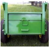
Trailer's box comes with a spring-loaded latch. When released, box manually tilts overcenter.
