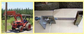
Dan Servideo recently used his loader-mounted post clamping device to pick up and place 8 5/8-in. sq. pressure-treated posts.
