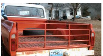
Dale Herigon used old galvanized water pipe to make this new tailgate for his pickup.
