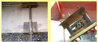
Double-nutted, 1-in. dia. threaded rod tightens device to bucket lip (left). A post holder with angle iron sides is then attached to threaded rod.
