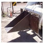
Narrow mini-bucket mounts on a skid steer loader, making it easy to fill a small cement mixer with just the right amount of aggregate.
