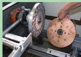
Mag-Trans unit consists of a copper disk driven by the DC motor running at its optimum rpm's.
