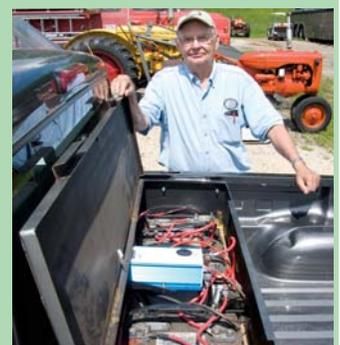
Located behind the pickup cab, the battery case comes with 10 deep cell, lead acid batteries which recharge in just 4 hours.
