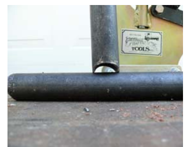
Tube Notcher (left) is designed to "V" out the end of a pipe in preparation for welding it to another pipe.
