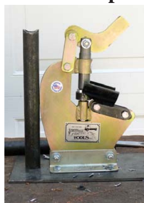
Tube Notcher (left) is designed to "V" out the end of a pipe in preparation for welding it to another pipe.
