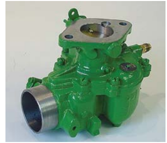
Gary Hoefling says his modified Zenith carburetor cleans up the black smoke and fouled spark plugs common to Deere 3010/3020 and 4010/4020 tractors.
