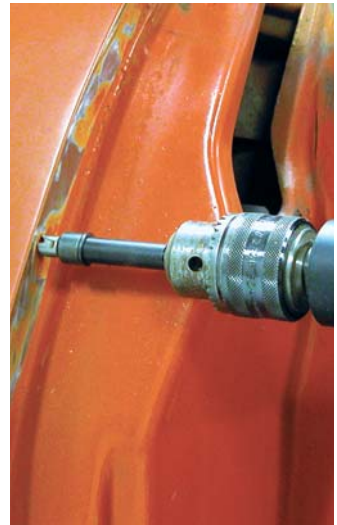
Spotweld cutter consists of an arbor with a pilot on it that helps line up the hole, and a cutter that screws onto arbor.
