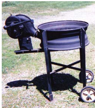
Alvin Oien made this forge out of a truck wheel rim and an antique hand-cranked blower. He uses it to make knives and parts for farm repairs.
