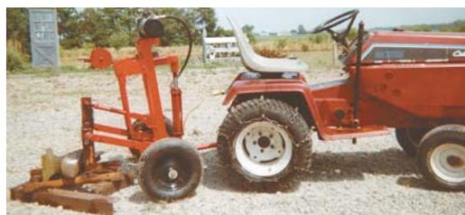
**William Hettler's Cub Cadet garden tractor has no hydraulics, so he built this 3-pt. "dolly" for it. Power is provided by a self-contained, 12-volt hydraulic power pack.**
