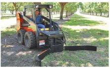
Skid loader-mounted "dirt hole closer" has a pair of 60-in. long, 10-in. high steel wings that open up 8 ft. wide.
