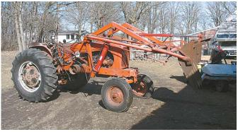
Using 2 by 4-in. rectangular tubing, some well casing and 1/2-in. steel plate, Don Ramberg built this light-duty loader for his Allis Chalmers WD tractor.
