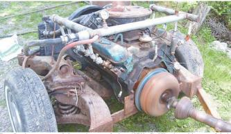
Dan Jamison converted the engine out of a late 1970's Cadillac into this powerful air compressor/sandblaster.
