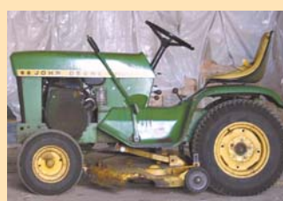
He cut off tractor's front spindles and then made extensions to widen them and lift the front end (left). He replaced the rear wheels with 28-in. high tires.
