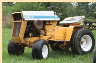
He started with a Cub Cadet 125 model (left). He stripped tractor down to the frame, which he lengthened by 3 1/2 in.
