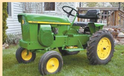
He cut off tractor's front spindles and then made extensions to widen them and lift the front end (left). He replaced the rear wheels with 28-in. high tires.
