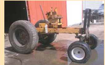
He started with a Cub Cadet 125 model (left). He stripped tractor down to the frame, which he lengthened by 3 1/2 in.
