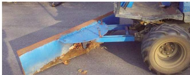
Home-built blade can be angled left or right by pulling a pair of pins and then manually moving blade.
