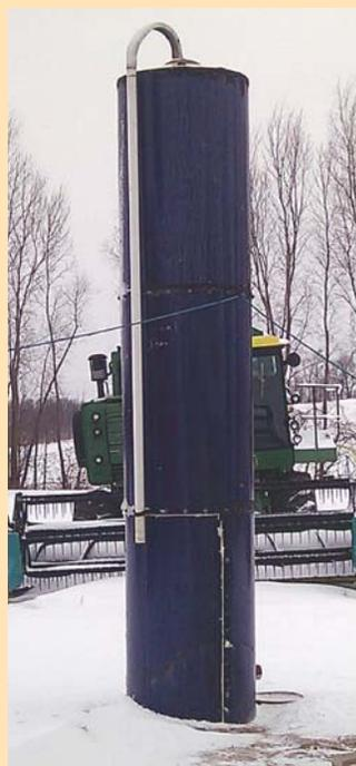
Mini sealed silo stands just 15 ft. high and 36 in. in dia. It's filled by a pipe with a gooseneck-shaped tube on top (left). Feed is augered out the bottom into a feed pan.
