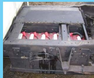
Remote control unit attaches to a lanyard Anderson wears around his neck (left). Truck is powered by twenty 6-volt, deep-cycle, lead-acid batteries stored under pickup bed.
