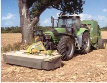
In addition to using a 30-ft. Claas rotary mower and then raking and baling with 2 Claas Uniwrap round silage balers, the Harbers also used a 10-ft. Claas mower on front of a tractor with a Deere baler on back
