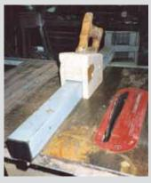
Merl Stangl, Atlantic, Iowa: "When using my table saw, instead of pushing the wood being cut with my hand I use a homemade wooden block that's designed to fit over the saw's guide bar. The handle off an old crosscut saw is screwed and glued into the block, which is made from 3/4-in. thick plywood and painted white. A side board extends down on each side of the block to the table saw's surface."
