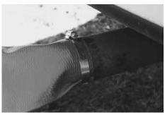
Rigid plastic adapter clamps onto vehicle's exhaust pipe.
