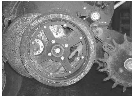
Open spoke design of new replacement gauge wheels keeps them free of mud.
