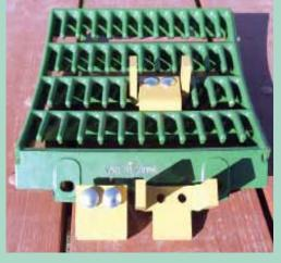
bar concave in the Deere STS rotor is that there isn't enough space between the round bars to let grain out," says Estes. "We have designed a new grate that has 7/16-in. square keys installed instead of the round bars, with a 1 1/2-in. space between them for 68 percent greater openings.'
