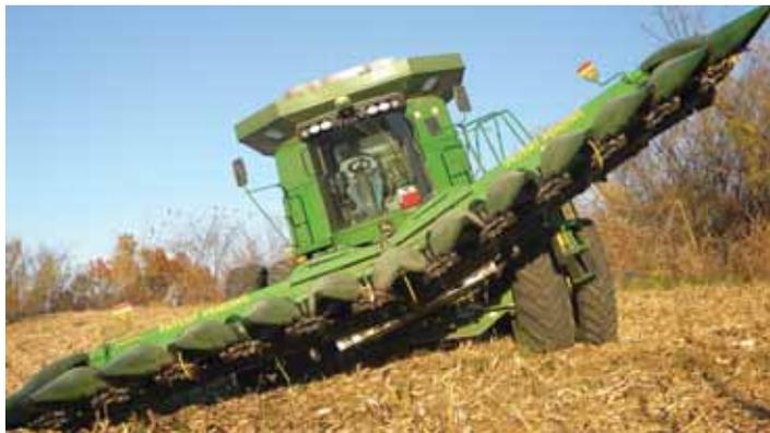
Split-Flex modified corn head pivots in middle. It can flex up or down 23 in. from level for a total of 32 degrees movement.
