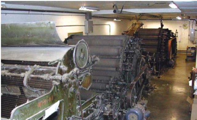
Equipment includes a 1907 carding machine and a 1920 spinning machine.
