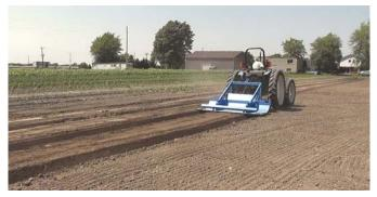
A machine called the Bedformer makes raised beds, allowing planting, cultivating, spraying and other tasks to be carried out with precision.
