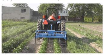
Skis mounted on front and back of cultivator has the sides of raised beds to allow precision work.
