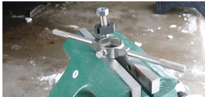
**Thread Chaser tool comes with a hinged die that wraps around the damaged bolt. A T-bar handle is used to quickly restore the threads.**
