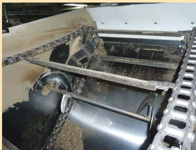
**A pair of chains with slats, combined with a 12-in. auger, are used to mix grain, protein, silage and chopped hay all together.**
