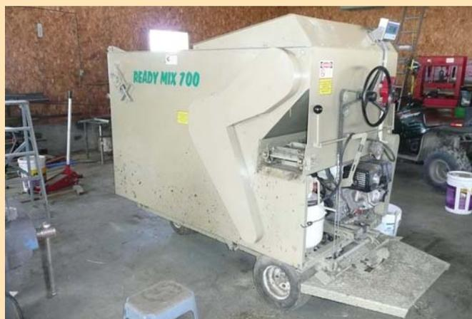
**Home-built, self-propelled feed mixer mixes and conveys feed to both sides of the machine.**
