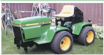
Edward and Eugene Kaban built this 4-WD articulated tractor using the front end of a Deere 300 garden tractor and the back end of a 316 model.
