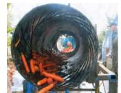
Water is sprayed onto vegetables as they feed through the rotating drum.
