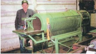
Belt-driven rollers turn the cleaner, with power supplied by a 3/4 hp electric motor.
