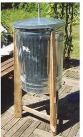
Home-built honey extractor fits inside a 31-gal. trash can that mounts on a 3-legged wooden stand.
