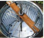
"Cage" with paired 1/4-in. dia. rods mounts inside trash can. Four honeycomb frames fit inside the paired rods.
