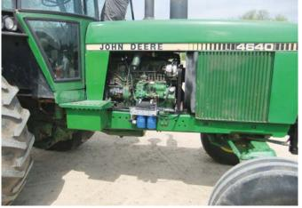
A Wisconsin company is selling the German-made Greasenergy conversion system, which allows diesel engines to burn straight vegetable oil.
