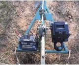
He mounted a winch on one side of boom and a 12-volt battery on the other side.
