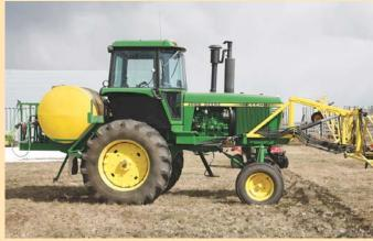
The 67-ft. boom is a 3-piece design that automatically folds back around the tractor, with 5-ft. breakaway tips at either end. By Jim Ruen, Contributing Editor
