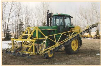
Robert Petrukovich converted a high clearance Deere 4440 tractor into this self-propelled sprayer, designing a mount that works like a front-end loader.
