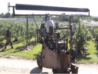
Tricycle rig was originally used to go over sweet corn with drop nozzles. Bartlett took the tank and booms off and built a rack to hold a roll of netting.
