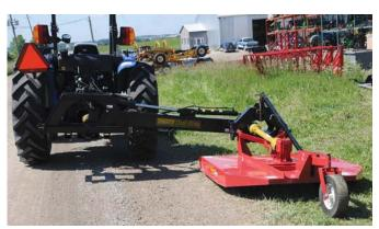
By extending or retracting a cylinder, mower can be tipped 90 degrees to cut nearly vertical bank.
