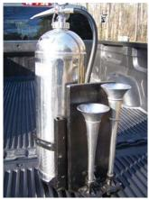
To scare away birds, Bill Jones made this loud air horn out of a 2 1/2-gal. fire extinguisher and a pair of air horns off an
